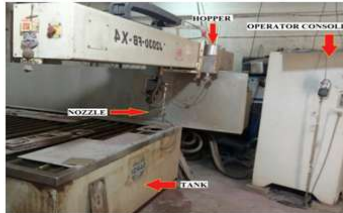
Input parameters and their levels for AWJM process. AWJM SETUP
