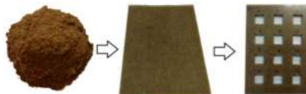
(a) Sundi wood dust (b) Prepared specimen (c) Machined specimen
